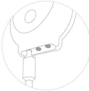
Insert the sensors jack into the base of the transmitter. Make sure you insert the sensor(s) jack first, then power on the Transmitter.
